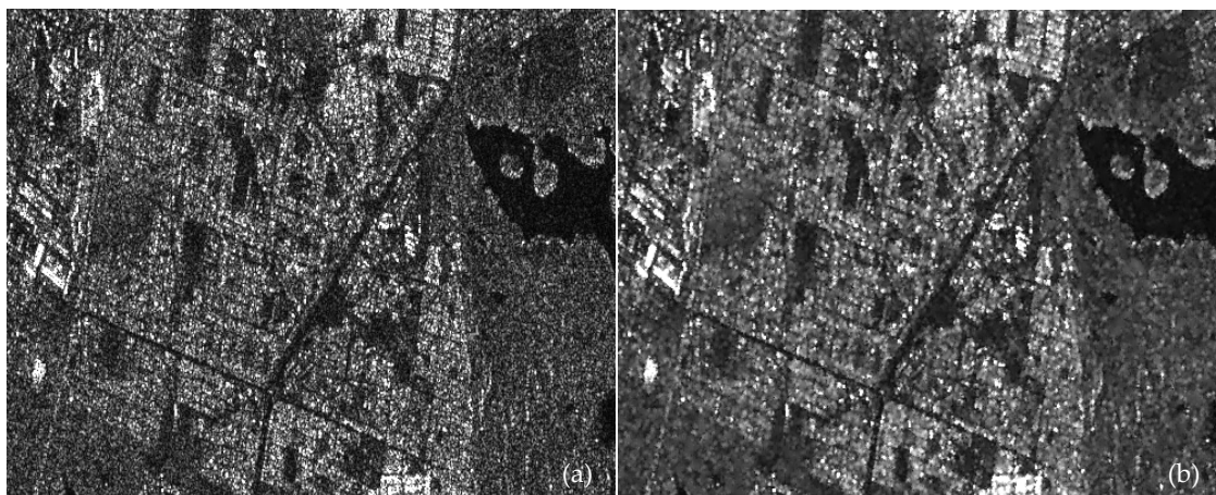
(a) unfiltered 1-look SAR image amplitude. (b) filtered SAR image amplitude obtained using the Complex-Gaussian-DE MAP filter for SLC SAR image ( cf. § 6.1).
