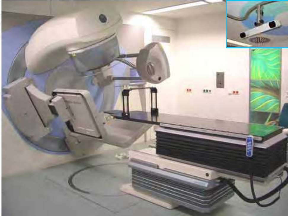
Figure 1. Linear accelerator installation at the University of Würzburg. The HexaPOD robot table is mounted on a standard treatment table. The MV treatment beam emerges through the gantry head, which in this picture is positioned at the top (ca. 340^\circ ). The MV EPID positioned opposite at the bottom (ca. 160^\circ ) records the radiation after it has passed through the patient and produces portal images. The kV X-ray source and corresponding flat panel, positioned at the right (ca. 70^\circ ) and left ( 250^\circ ), respectively, are rotated around the patient to produce cone-beam CT images. The inset on the top right depicts the tracking camera, which tracks the reflectors on the c-shaped bridge (see also Figure 2)
