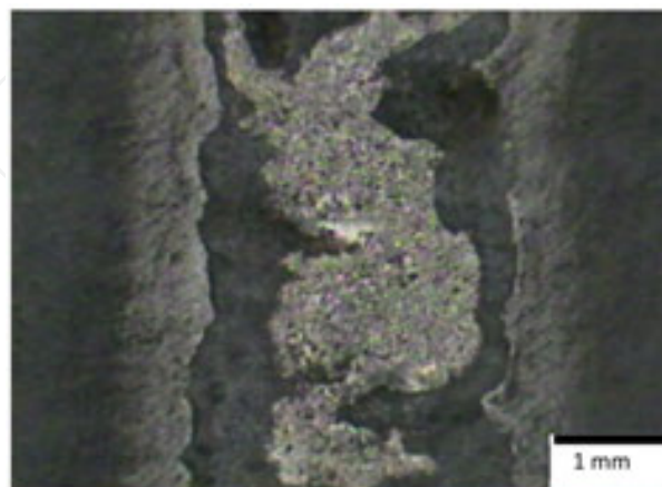
Figure 8. 32CrMoV12-28 steel alloyed with \text{Si}_3\text{N}_4 powder, laser power 1.2 kW
