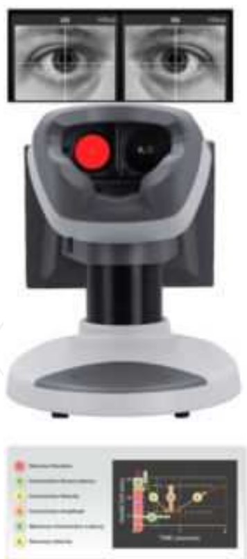
Figure 17. RAPDx (Konan, USA) measures Relative Afferent Pupillary Defect
