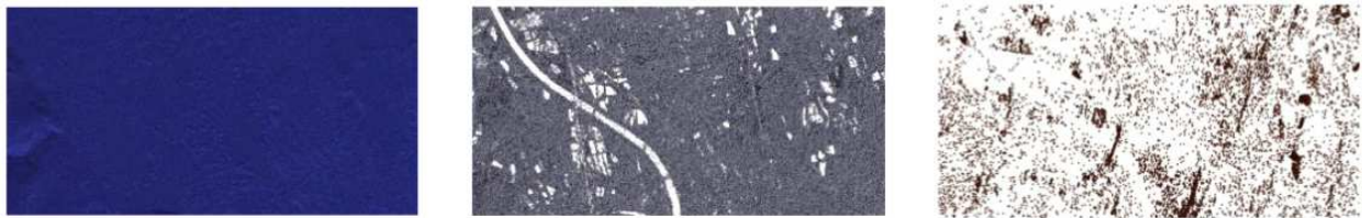
Figure 20. Breakdown of a subset of Figure 19 between: grid-based matching points (left), feature-based matching points (center), edge-and area-based matching points (right).
