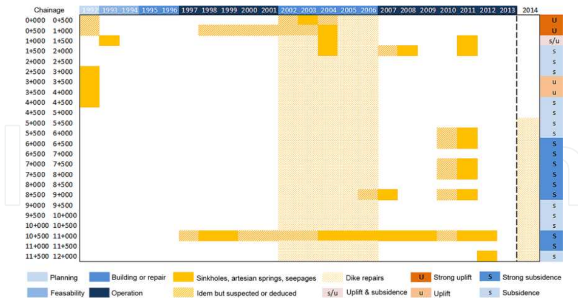
Figure 13. Comparison between sequences of hazard events along dike 18 and a qualitative assessment of the ground deformations computed from 1992 to 2010 with SBAS technique [36-38] ("SBAS" module of Sarscape software).
