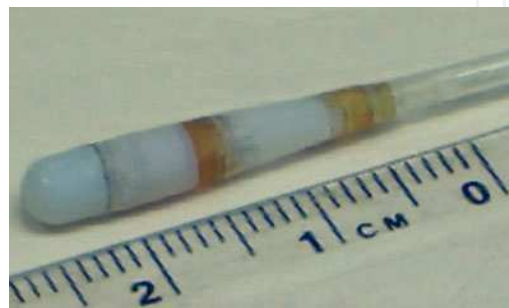
Figure 14. Ablation catheter with tri-axial force sensor
