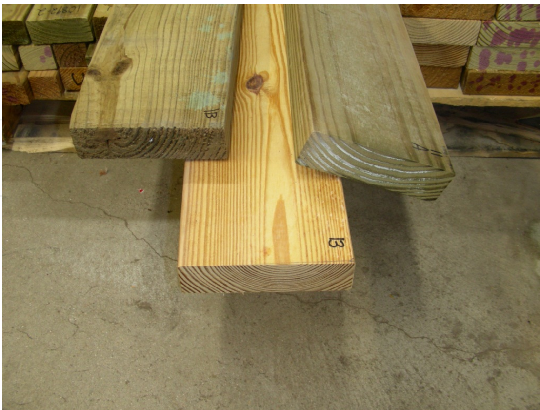
Figure 3. (From left to right) Wood treated with MCQ, DDAC, and ACQ. Cupric ions from the wood preservative cause the dark coloration of the wood. Excess copper has deposited on the MCQ (green splotches) and the ACQ (along the end grain) samples. SCALE: The boards are approximately 38 x 140 mm.
