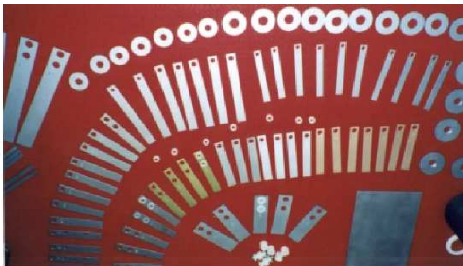
Figure 9. Coupons to measure corrosion.
