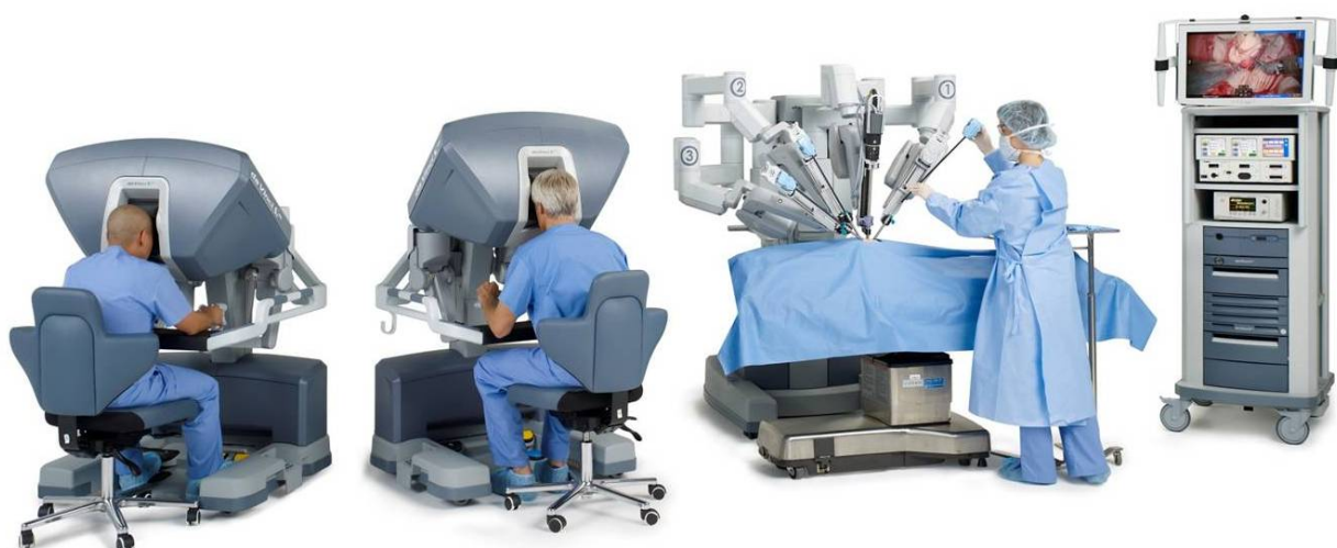
Figure 2. [26] : showing robotic and vision carts and the surgeon's console with an additional teaching console
