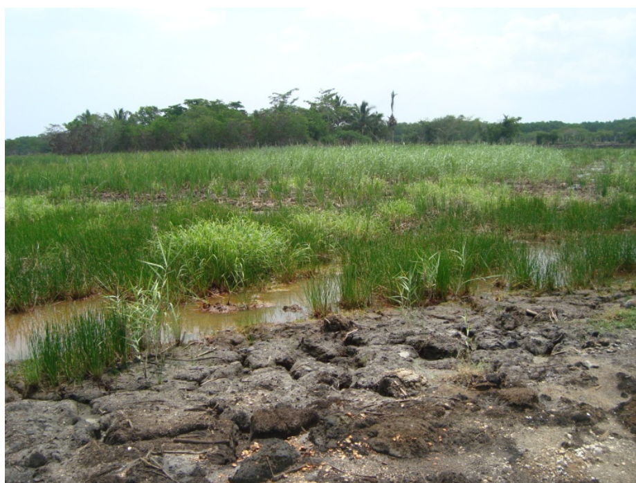
Figure 3. Formation of macroaggregates in soil with 12,155 mg.kg -1 TPH weathered.
