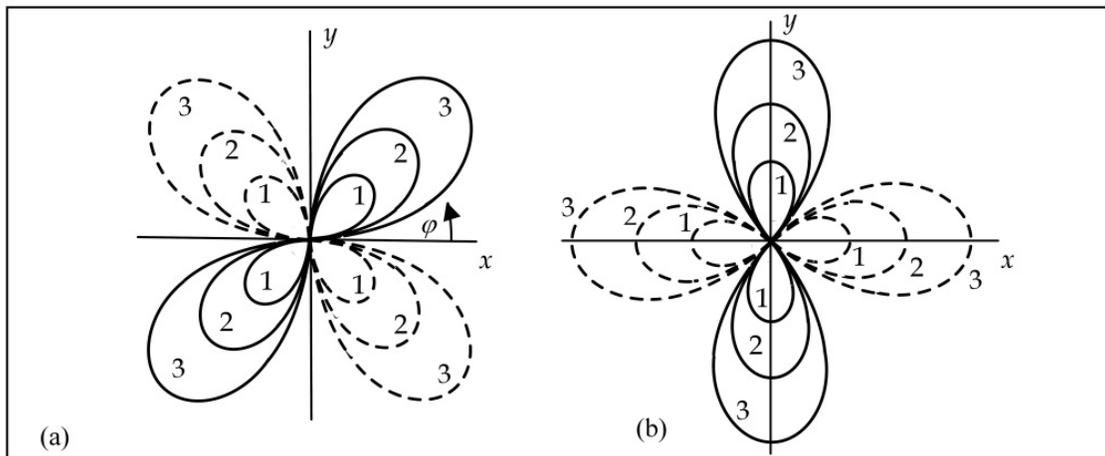
**Figure 1.** Polar diagrams of the electric potentials (a)  $\phi_{l,t'}(\varphi)$  and (b)  $\phi_t(\varphi)$  at  $\theta = \text{const}$  in the vicinity of the  $(0, 0, 1)$  direction in a cubic piezoelectric crystal. Numbers 1, 2, and 3 refer to the angles  $\theta_1 < \theta_2 < \theta_3$ ; solid and dashed lines relate to the potentials of different signs.
