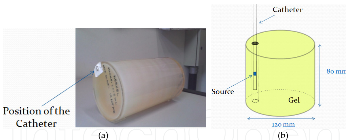
Figure 3. Cylindrical phantom to obtain the PDD curve: (a) with the MAGIC-f gel and (b) scheme of the irradiation setup.
