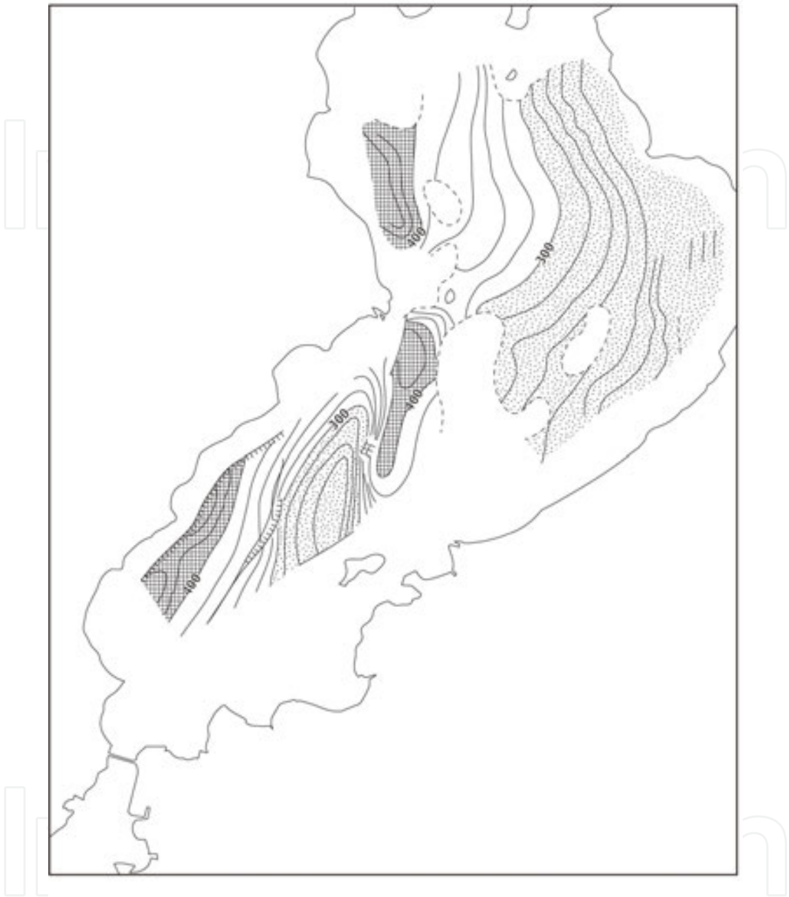
Figure 9. Active structure revealed by horizon A (Boundary of T and S bed) since about 0.43 Ma) of the seismic reflection survey [19] Meshed part: depth of A horizon more than 400 m, Dotted part: depth of A horizon lower than 300 m
