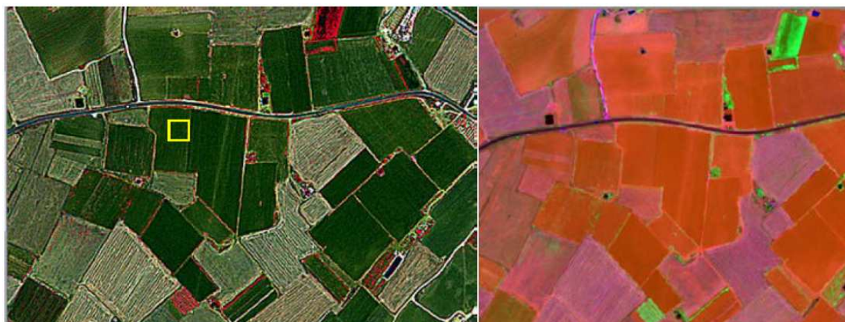
Figure 15. IKONOS 3 x 3 high pass filter (left) and PCA analysis (right)
