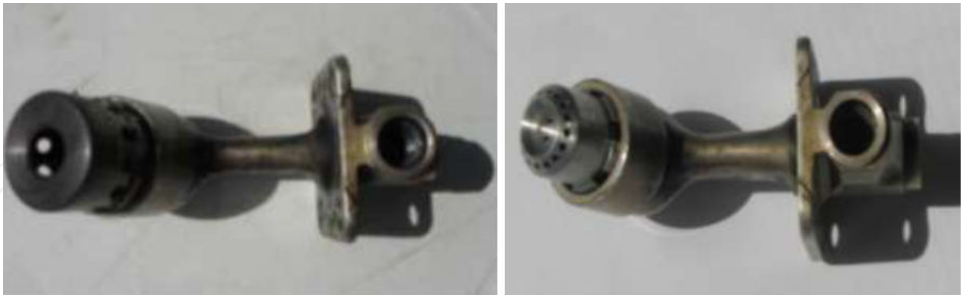
Figure 9. Injectors for liquid fuel for TV2-117A (left) and landfill gas for TA2 bio (right) [2]
