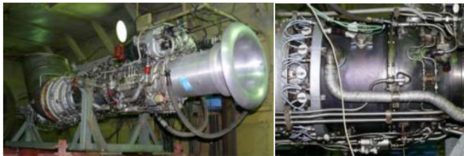
Figure 7. TV2-117A gas turbine (left) with detailed combustion chamber area (right)
