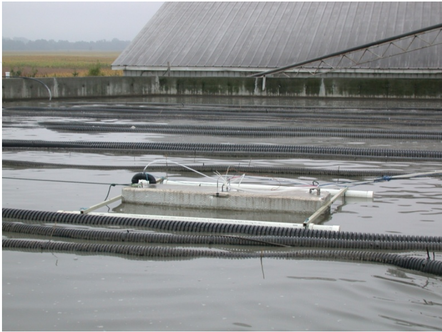
Figure 2. IRDA sampling device on a manure storage tank
