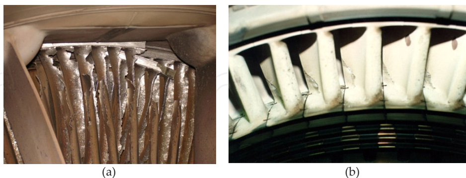
Figure 1. (a) FOD effects, (b) Turbine nozzles with deposits.
