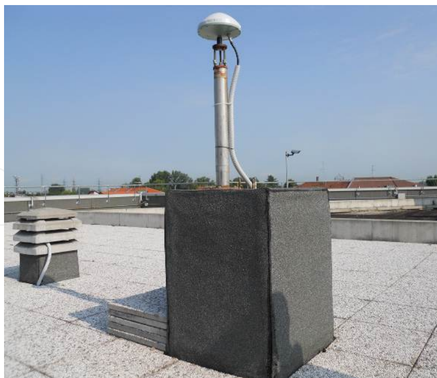
Figure 6. Pillar and antenna used for the NRTK test (VERC station)
