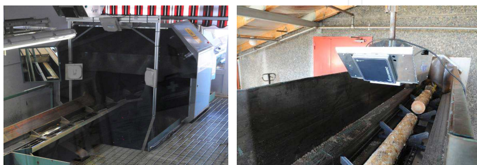
Figure 10. RFID readers in the log sorting and sawing in a saw mill.
