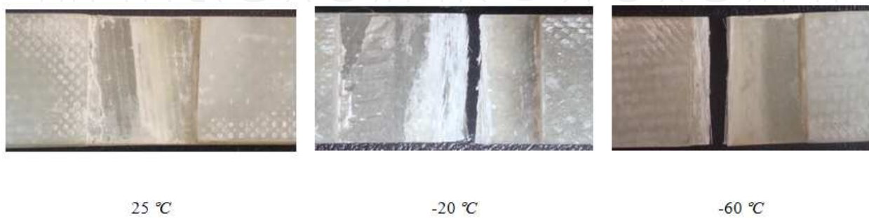
Figure 11. Failure regions of the composite specimens at different temperatures in transverse direction under compressive loading
