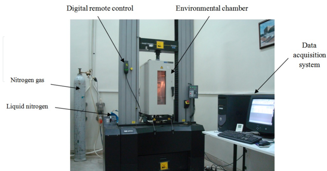
Figure 1. Experimental setup for mechanical tests at both room and low temperatures
