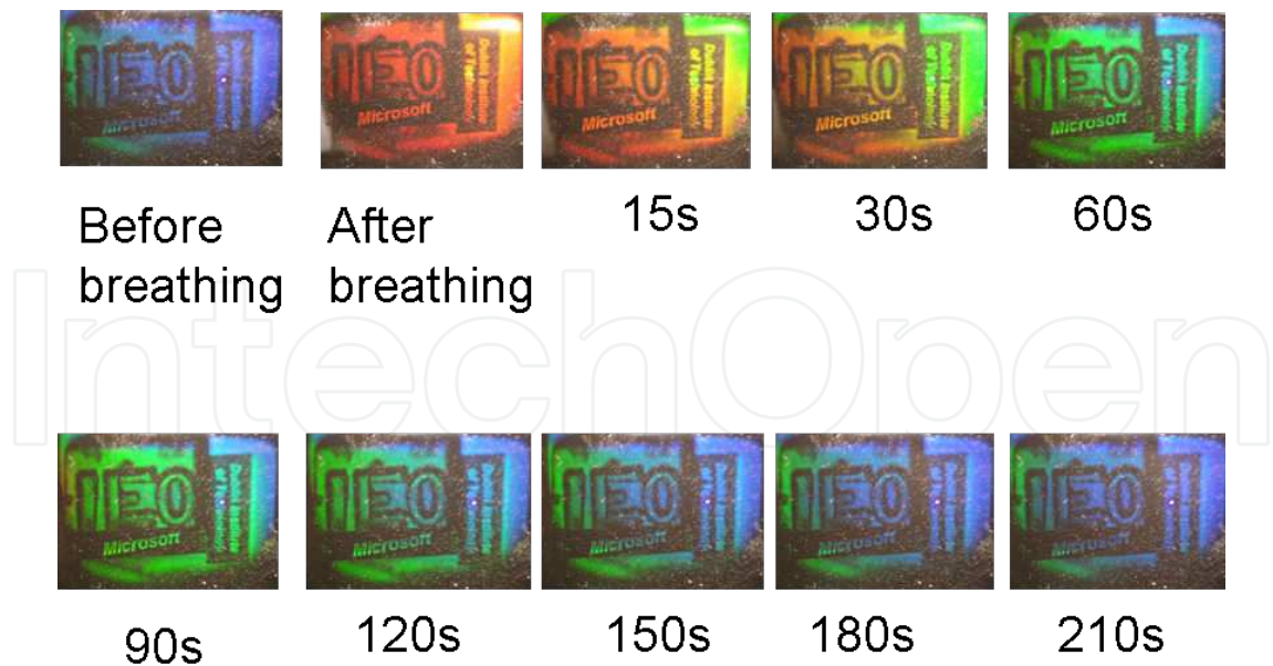
Figure 1. Moisture sensitive colour changing hologram
