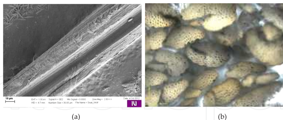
Figure 8. a) Longitudinal view (2500x magnification) and b) cross-section of sisal fibre
