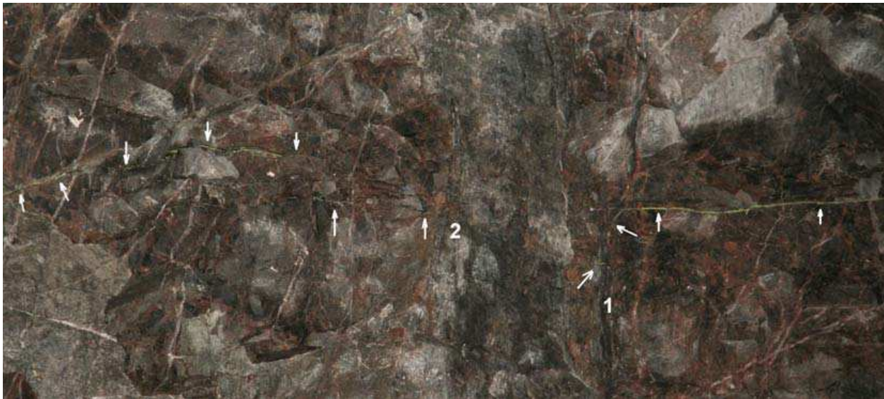
Figure 7. Hydraulic fracture (green plastic) crossing a shear zone on the face of a tunnel excavated through the fracture. "The arrows indicate the trace of the fracture with green plastic contained in it. There is no clear fracture between points 1 and 2 but the fracture may have crossed this zone either deeper into the rock or in the rock that has been excavated. Approximately 2 m of fracture extent is visible" (Jeffrey et al., 2009).
