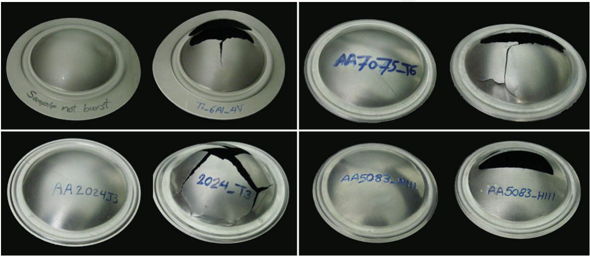
Figure 10. Burst and not burst samples of Ti-6Al-4V alloy
