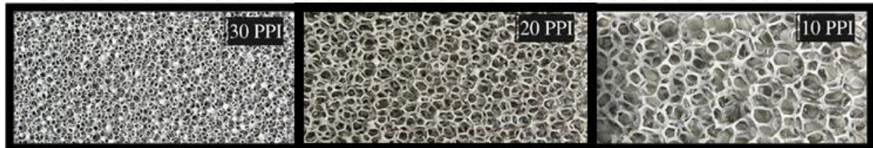
Figure 7. Metallic foam of different pores per inch.
