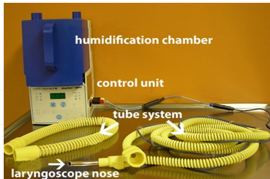
Figure 15. Device for moistening and warming-up of the respiration gas. The central unit (white) incorporates the electronical control unit. The humidifying chamber (blue) for single or multiple use is fixed at the central unit. The tubing system (yellow) is splitted in a short tube which transports the ventilation gas coming from the respirator to the humidifying chamber, and in a long tube which transports the now moistened and warmed-up gas from the humidifier chamber to the jet laryngoscope. The distal part of the long tube is metallic and is connected to the jet laryngoscope.
