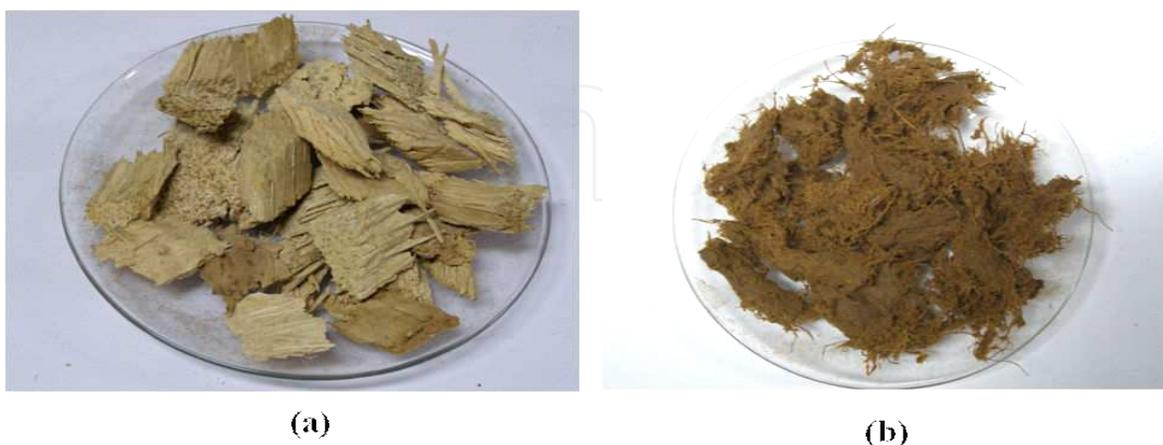
**Figure 2.** Oil palm trunk chip (a) and steam exploded oil palm trunk pulp (b)
