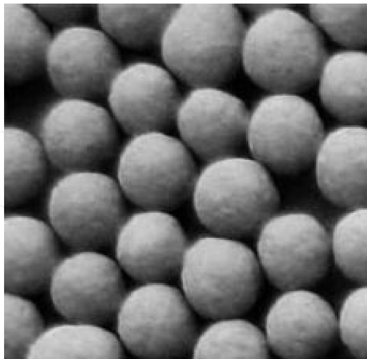
Figure 4. Bauxite, sphericity \sim 0.90 – Photo courtesy: Oxane.
