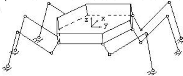
Figure 6. The simplified structure model of hexapod walking robot
