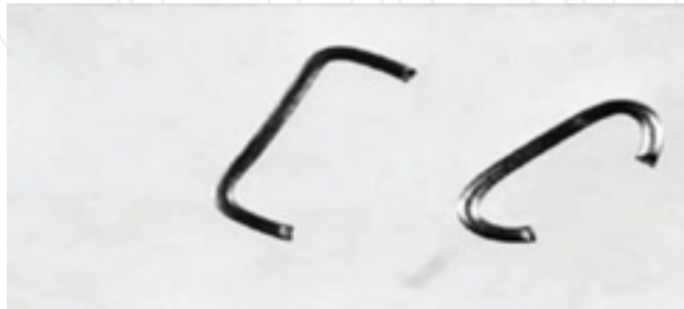
Figure 4. Medical staple before and after distraction (Laster, MacBean et al. 2001)
