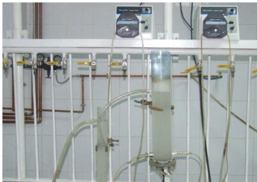
Figure 4. Laboratory simulation of aerobic sewage treatment
