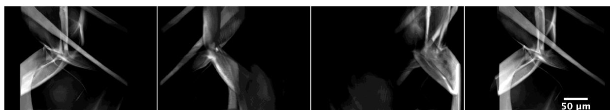
Figure 12. Three-dimensional rendering of a macro-porous cellulose structure in a wet state, observed from different angles. The sample was stained with Calcofluor White (CFW) before imaging.
