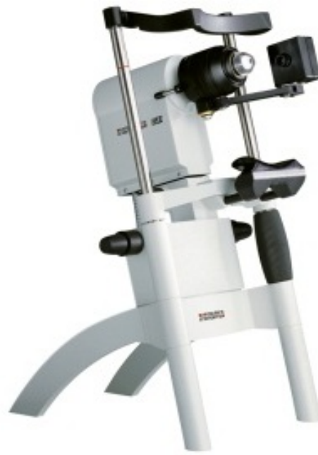
Figure 1. Heidelberg Retina Tomograph 2 Rostock Cornea Module The device uses a 60x water-immersion objective lens (Olympus Europa GmbH, Hamburg, Germany) and utilizes a 670-nm diode laser as the light source with the area of observation 400 \mu m square section.
