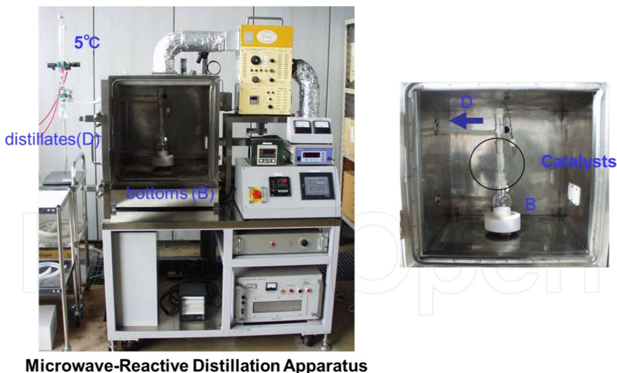
**Figure 12.** Microwave apparatus for preliminary studies on reactive separation for ETBE synthesis
