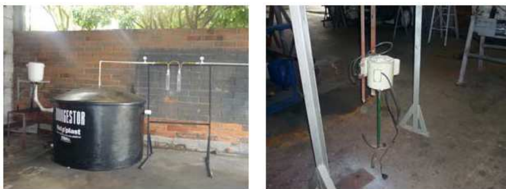
Figure 3. Installation of bioreactor and equipment to trituration
