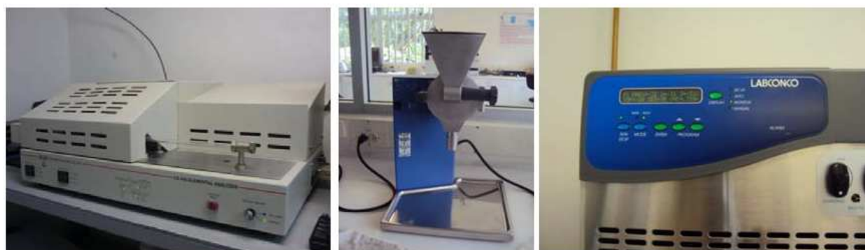
Figure 2. Elemental analyzer CE – 440 (a), Crusher MF Basic- IKA WERKE (b), Lyophilizer LABCONCO - Freezone 12L (c).
