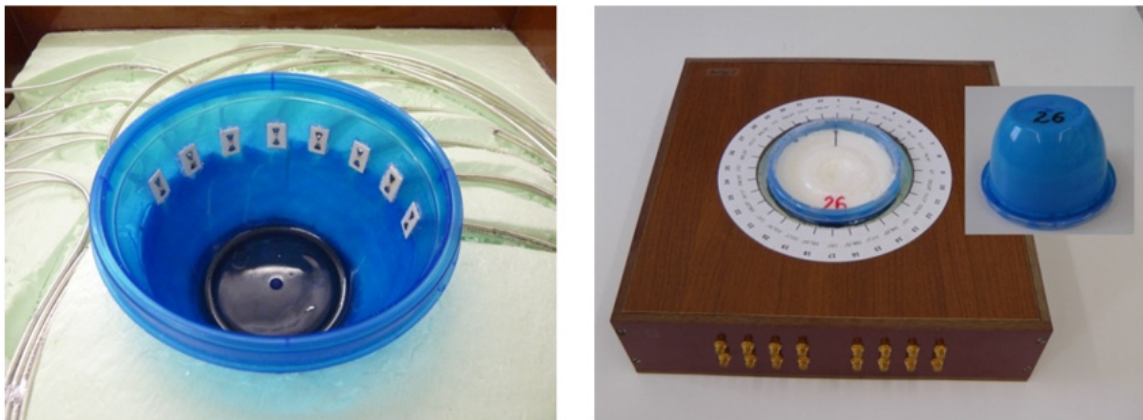
Figure 50. Antenna array: Assembly stage before casting the contact layer. The connected and affixed differential fed antennas and the container for the outer boundary of the contact layer are still visible (left panel). Finished antenna array with inserted rotatable breast phantom (right panel)
