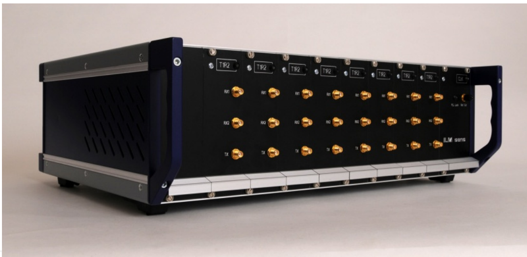
Figure 4. 8 Tx-16 Rx MIMO radar for microwave breast imaging (operational band 20 MHz – 6 GHz; 9 th order M-sequence, USB2 interface). M-sequence units (as shown in Fig. 6 of Chapter 14) and RF-front ends are separated to get more flexibility for experimental purposes.
