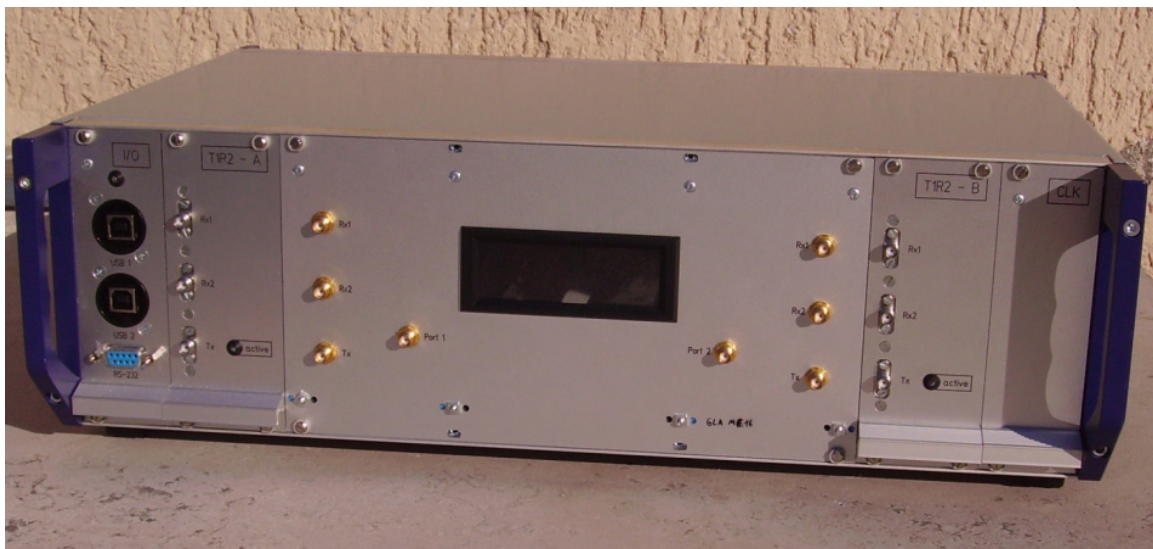
Figure 2. M-sequence two-port network analyzer (operational band 40 MHz – 8 GHz, 9 th order M-sequence, USB2 interface). It can be extended by an RF-switch matrix for MIMO-radar imaging.
