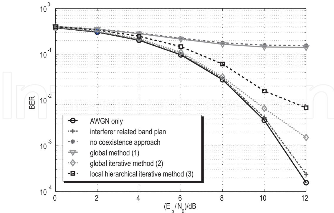
**Figure 22.** BER vs.  $E_b/N_0$  for AWGN and fixed SIRs of -10 dB (IEEE 802.11a WLAN [47]), 0 dB and 5 dB (IEEE 802.15.3a MB OFDM UWB 1 and 2 [2]) regarding an interferer related band plan, no coexistence approach and the coexistence approaches 1 to 3 [12].
