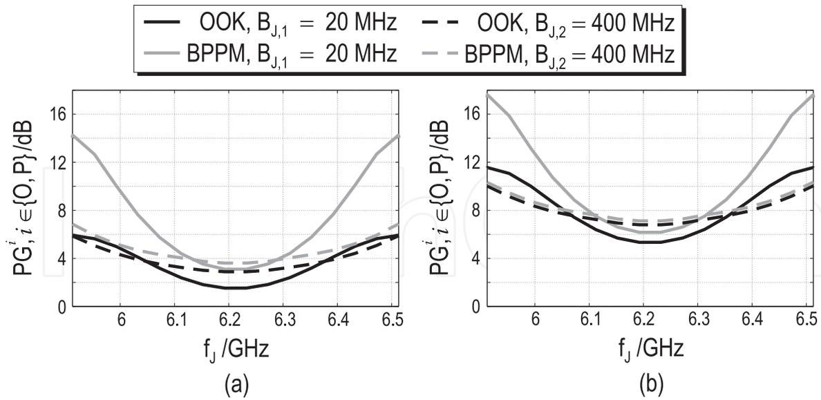
**Figure 19.** Processing gain of an OOK and BPPM specific energy detection vs.  $f_j$  for  $\text{SINR}_E = 0$  dB,  $\text{SNR} = 10$  dB,  $B_{J,1} = 20$  MHz,  $B_{J,2} = 400$  MHz and  $T_{b,J} = 102.4$  ns for  $T_b = 2T_p$  (a) as well as  $T_b = 4T_p$  (b).
