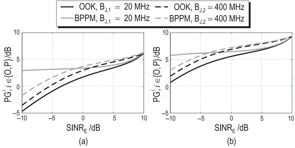
**Figure 18.** Processing gain of an OOK and BPPM specific energy detection vs.  $\text{SINR}_E$  with  $B_{J,1} = 20$  MHz and  $B_{J,2} = 400$  MHz,  $f_J = f_c + 50$  MHz,  $\text{SNR}_E = 10$  dB,  $T_{b,J} = 102.4$  ns,  $d_J(B_{J,1}) = 0.4883$  and  $d_J(B_{J,2}) = 0.0244$  for  $T_b = 2T_p$  (a) and  $T_b = 4T_p$  (b).
