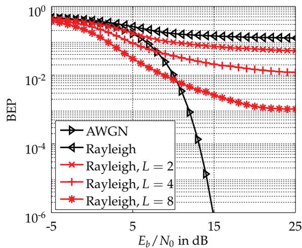
Figure 16. BEP in the *Rayleigh* channel with SLS
