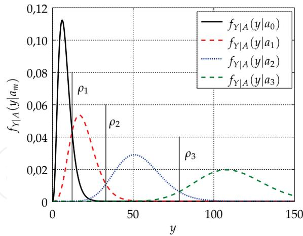
Figure 5. Optimal interval thresholds for 4-PAM ( $\gamma = 10$  dB)
