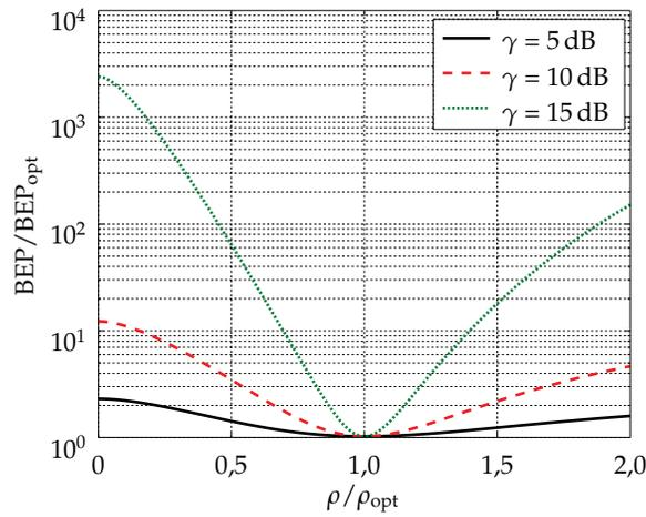
Figure 6. Sensitivity of the BEP related to the interval threshold  $\rho_1$  for OOK
