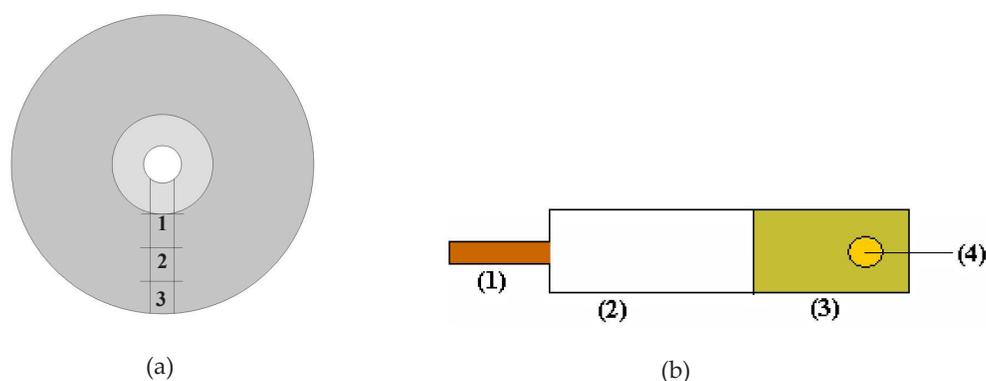
**Figure 1.** Regions of CD-Rs: (1) inner, (2) central and (3) out border. (B) CDtrode: (1) electric contact of copper, (2) PTFE tape to fix the electric contact, (3) 1KFA25 Kapton tape<sup>®</sup> applied on the surface to delimit the area of the electrode, and (4) area of the working electrode [29].
