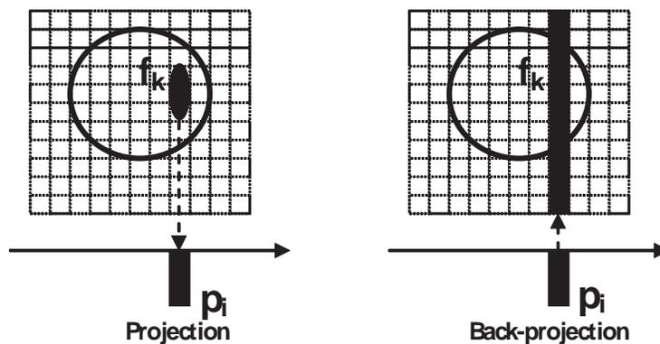
**Figure 7.** Illustration of projection and back-projection processes.
