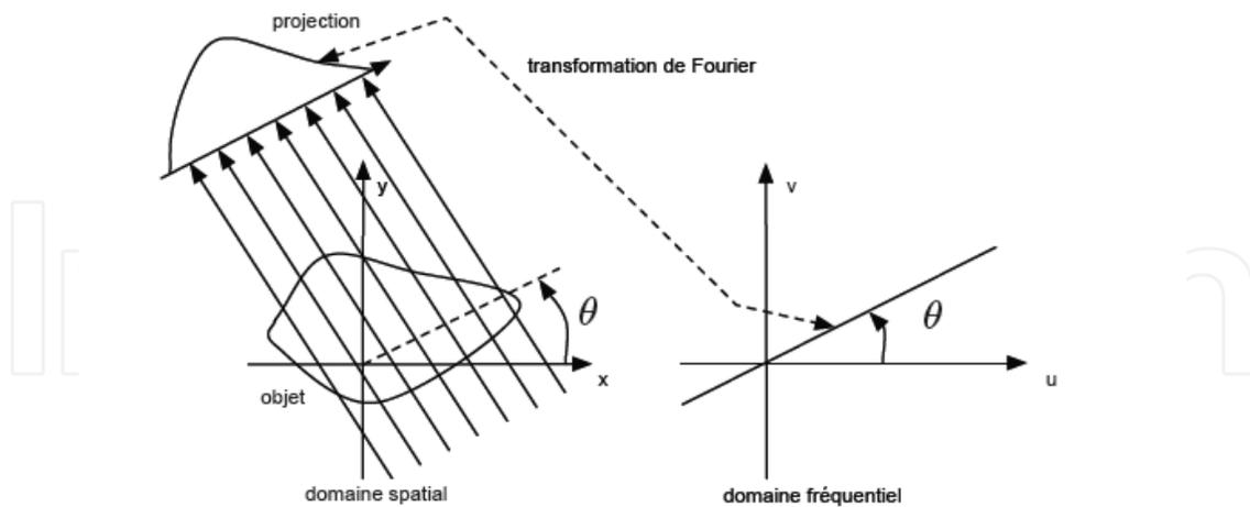
Fig. D.2. Illustration of Central Slice Theorem of Fourier.
