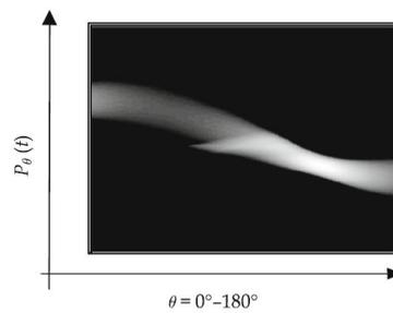
**Figure 5.** Example of projection Sinogram of the object of Fig. 4: the y-axis shows the projections (gray level variation as a function of the pixel's or detector's position) and on the x-axis, these one pixel width projections are arranged from the first projection ( $\theta=0^\circ$ ) to the last one ( $\theta=180^\circ$ ). Each sinogram will be used for the reconstruction of one pixel layer of the object.
