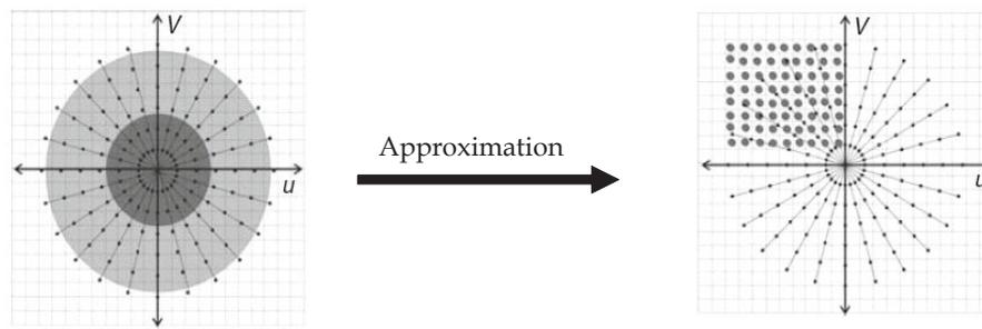
**Figure 3.** Fourier transform of a projection  $P_\theta(t)$  (left) and the interpolated data in the square coordinates system (right). The interpolation of high frequencies (high values of  $(u, v)$ ) is inaccurate.
