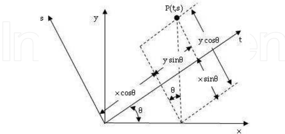
Fig. D.1. Considered coordinates system: fixed (x, y) and rotational (t, s), used to identify a projection point P of the object.
