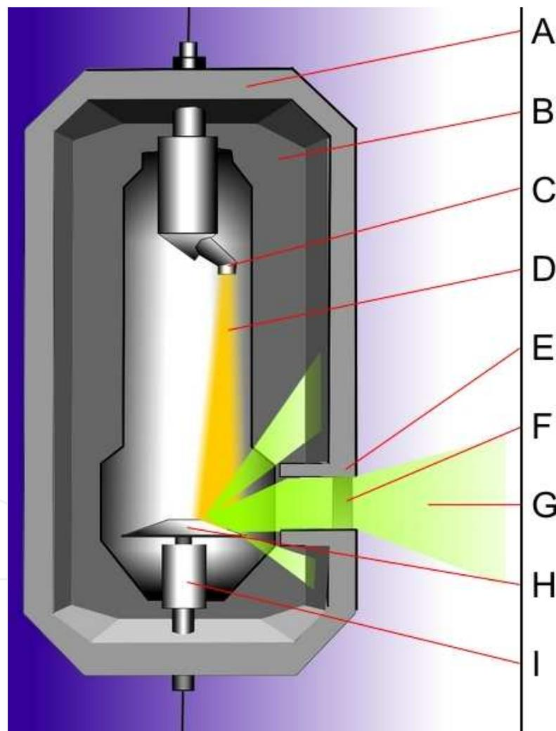
**Figure 1.** The x-ray tube. Legend: A – housing; B – oil bath for cooling; C – cathode; D – electron beam; E – collimators; F – filters; G – x-rays; H – anode; I – engine for anode rotation (illustration: J. Čaluk).
