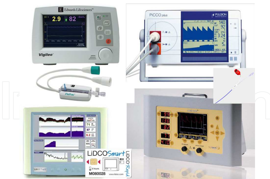
Figure 10. Four main pulse contour monitors being used. FloTrac-Vigileo (top left), PiCCO with femoral artery catheter that provides transpulmonary thermodilution (top right), LiDCO with user card (bottom left) and PRAM-MostCare (bottom right). LiDCO system also provides lithium dilution cardiac output. (Images downloaded from manufacturers websites)
