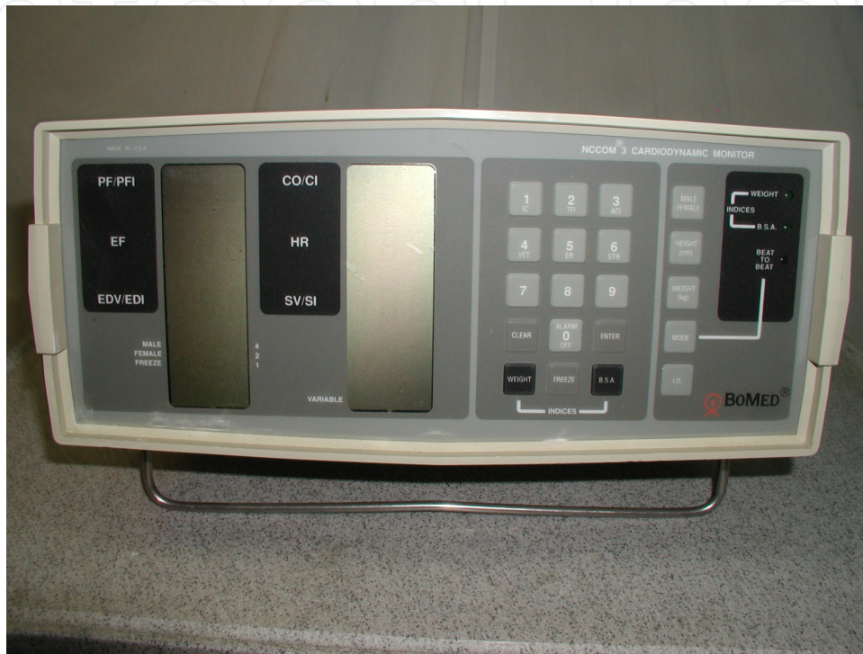
Figure 1. The BoMed NCCOM3. It connects to the patients using eight skin surface electrodes applied to the mid-neck and lower chest at the level of the diaphragm. Two additional ECG electrodes can be added. The BoMed is calibrated by inputting the patient's height and weight. Cardiac output and related bioimpedance variables are displayed as numbers. Data is averaged over 16 heart-beats.
