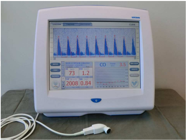
Figure 9. USCOM monitor showing Doppler signal data on its screen. The flow profiles are automatically outlined to measure stroke volumes. Below numerical readings are displayed. Lower right is a trend plot of saved cardiac output readings. The hand held USCOM probe is shown in front of the monitor. Ultrasound gel is applied to the probe to improve its acoustic contact.
