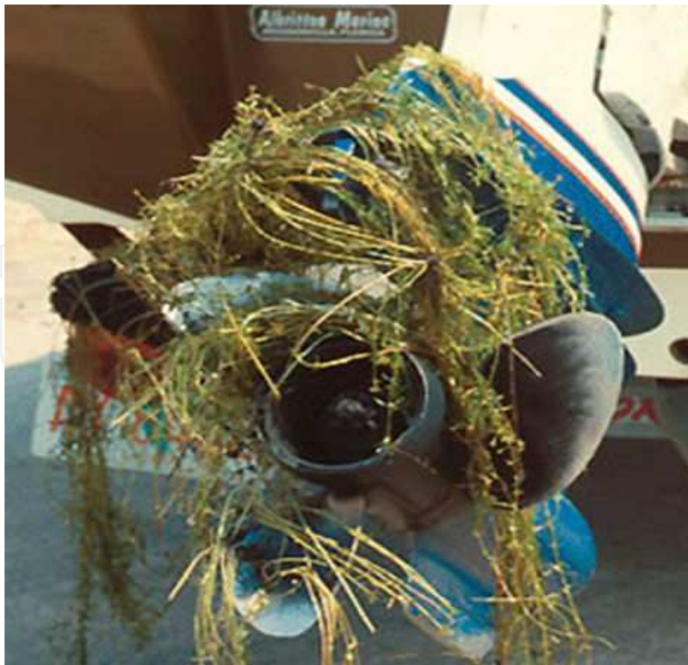
Figure 4. Boat motor clogged with hydrilla. Photo courtesy UF/IFAS Center for Aquatic and Invasive Plants.
