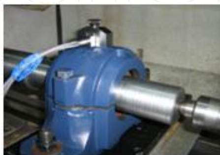
Figure 6. AE sensor mounting on the bearing housing with a magnetic clamp
