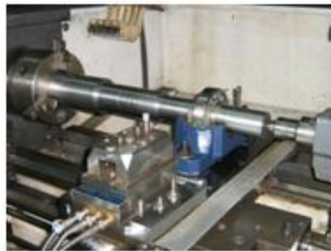
Figure 4. Shaft, test bearing, and the housing arrangement on the lathe machine
