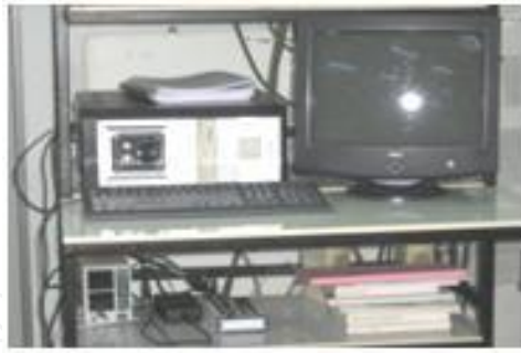
Figure 7. Instrumentation apparatus: PCI DAQ card, Connector block, and DC power supply
