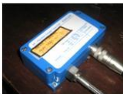
Figure 9. AE Piezotron Coupler Data Acquisition and Processing
