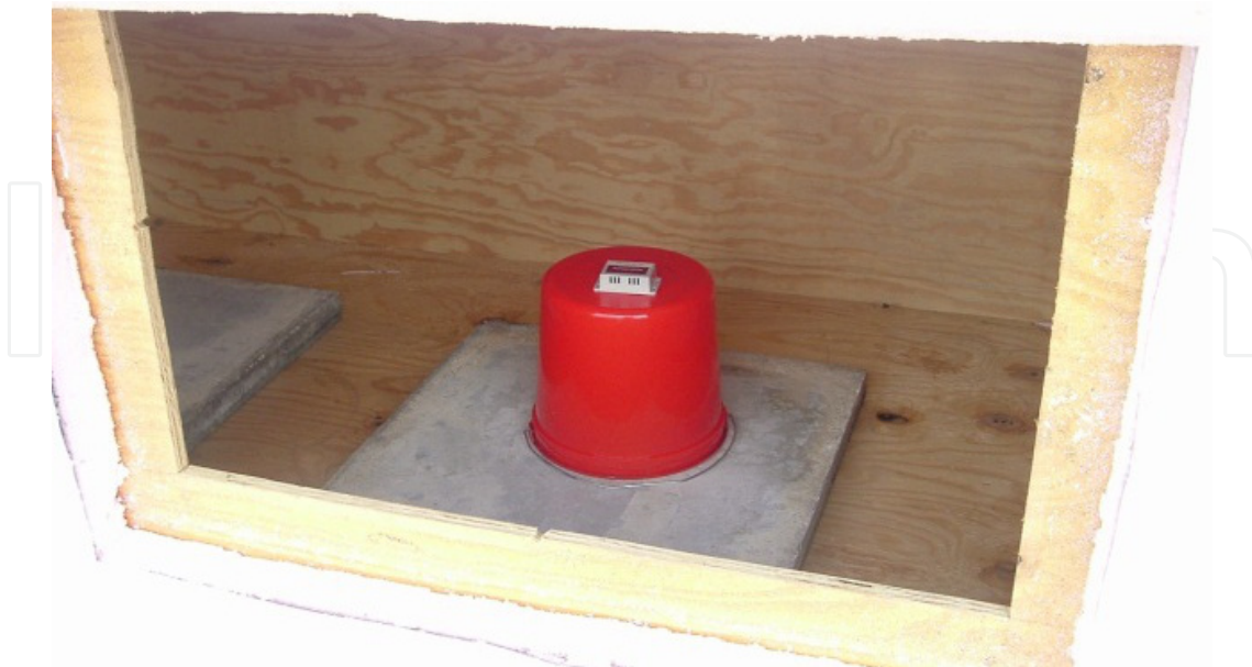
Figure 3. Mini-roof system showing temperature sensor installed inside a mini-roof.
