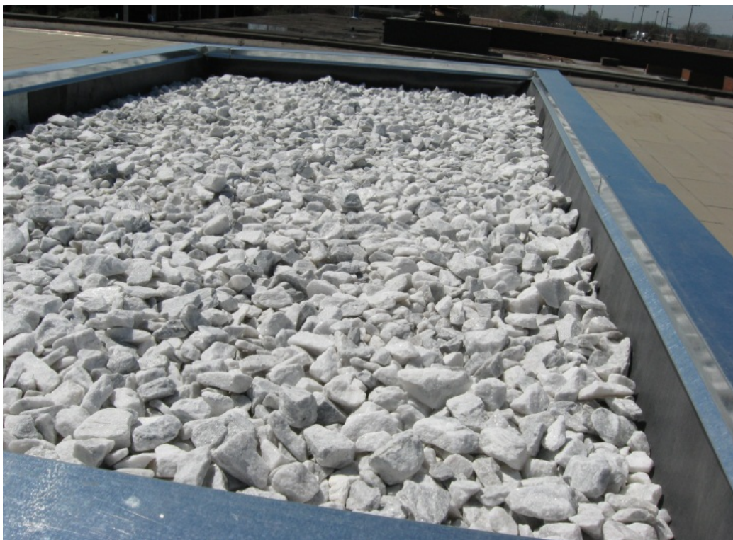
Figure 8. Mini-roof equipped with crushed marble chips.
