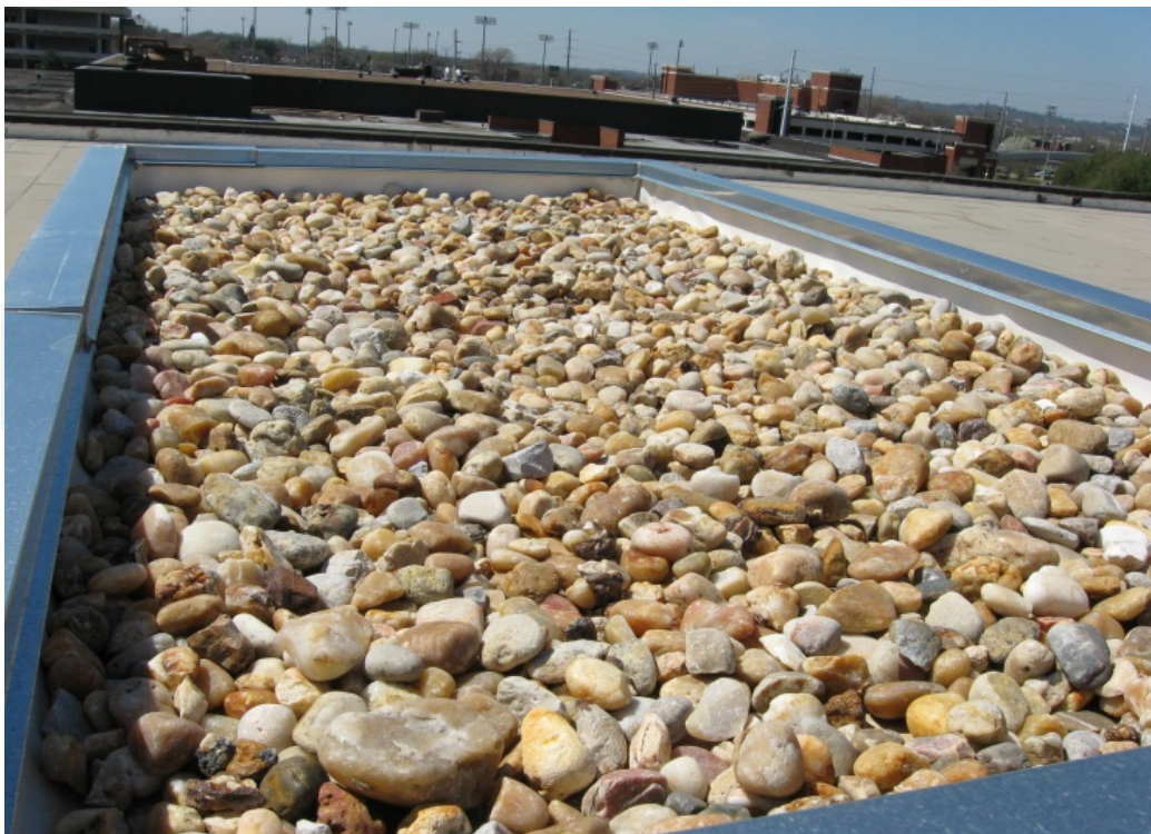
Figure 7. Mini-roof equipped with river rocks.
