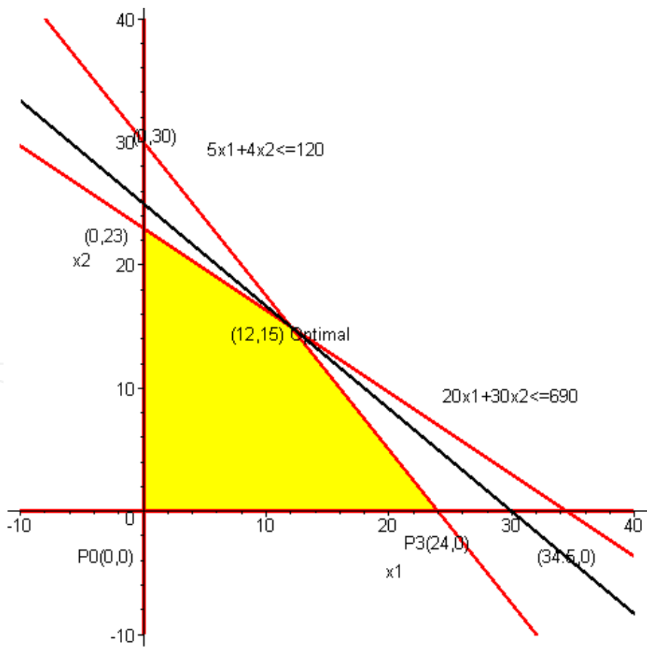
Figure 5. The set of points satisfying the constraint of this linear programming problem (the convex set as a shaded region)
