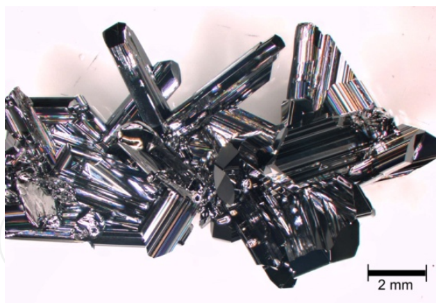
Figure 30. Crystal of \text{ZrAs}_2 grown by chemical vapor transport.
