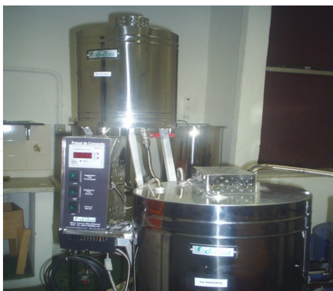
Figure 9. Small plant for the production of biodiesel
