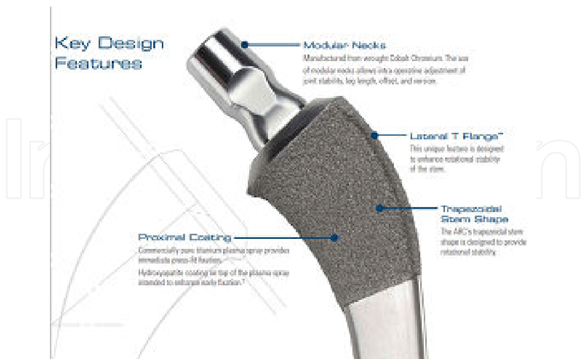
Figure 16. Key Design Features of the ARC™ stem.
