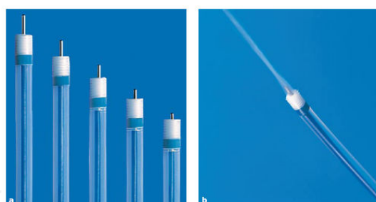
Figure 7. Flush knife (DK2618JN10–30; Fujifilm Corp.). a The appropriate length of the needle can be selected from among 1, 1.5, 2, 2.5 and 3 mm sizes. b Water jet function through the knife sheath.
